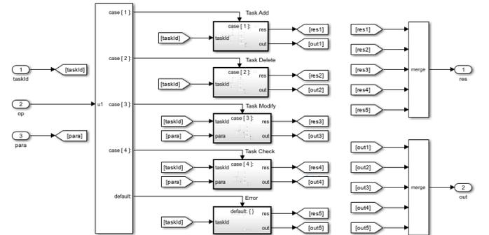
Fig. 1. An example of model with complex internal states. This is an AutoSAR CPU task dispatch model. It mainly contains the four operations of adding, deleting, modifying and checking CPU task in the queue.
