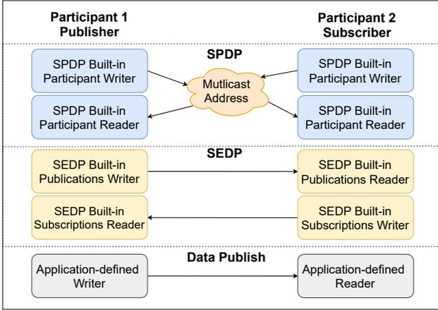
Fig. 2. A simplified example of an RTPS publisher and a subscriber, involving the state of SPDP and SEDP, and Data Publishing.
