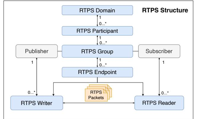
Fig. 1. Entity structure of RTPS protocol.
