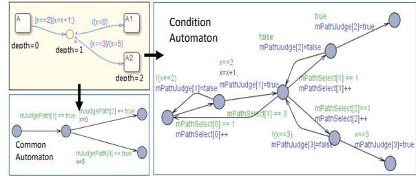
**Figure 4: The common and condition automata for a composite state transformation, capturing internal transition.**
