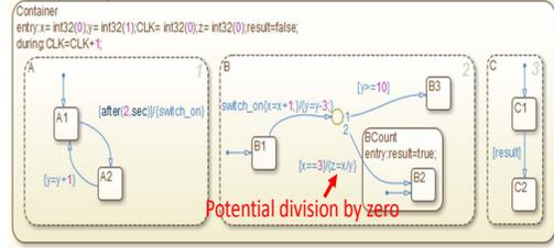
Figure 6: Manual model for validation testing
