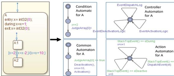
**Figure 3: The controller and action automata for a composite state transformation, capturing activation and deactivation.**
