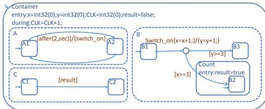
Figure 1: A Stateflow example for counter task which covers most advanced modeling features.
