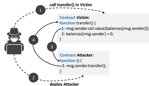
Figure 1: A simplified scenario of DAO attack.
