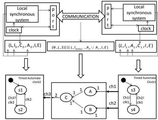
Figure 1: Modeling framework for multi-clock embedded systems with heterogeneous behaviors.
