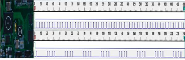
**Figure 5: The left side of the figure is our implemented experiment platform of the control system. The right side are the results run-time comparison for different design, 58, 33 pulses sampled for 24 MHZ, 12 MHZ, respectively.**
