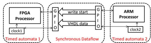
Figure 4: An abstraction model of the function that initialize the card with the device configure information. ARM will pass those data to the FPGA.
