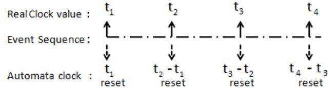
Figure 2: The mapping mechanism from the real clock value to the action of local clock in the timed automata to ensure synchronous reaction behavior.
