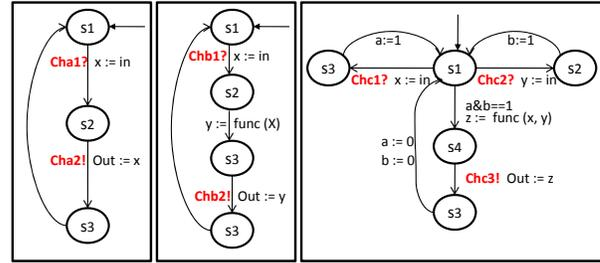
Figure 3: The translation from the synchronous dataflow to the timed automata.
