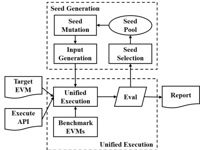
**Figure 1: Overall workflow of EVMFuzzer, which mainly includes the seed generation module for guided contract generation and the unified execution module for information collection and cross-checking.**
