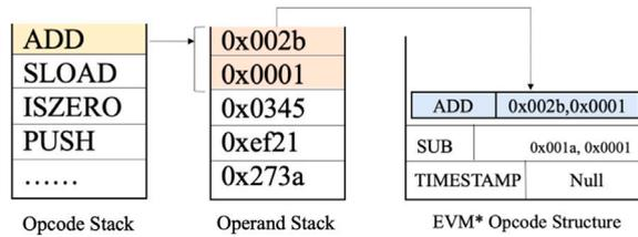
Fig. 3. The stack opcode structure of EVM\*. Each element of the code is the combination of the opcode and its operands.
