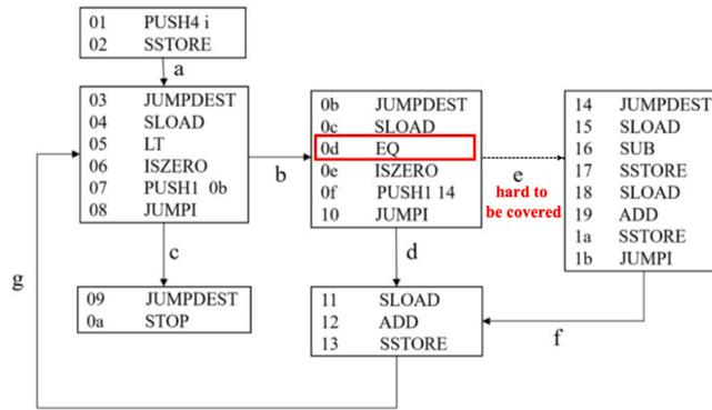
Fig. 1. The control flow of function *reward* on bytecode code level. According to the result of the opcode ‘EQ’, the branch e is hard to be covered by dynamic testing tools which leads to a false-negative of the tools.
