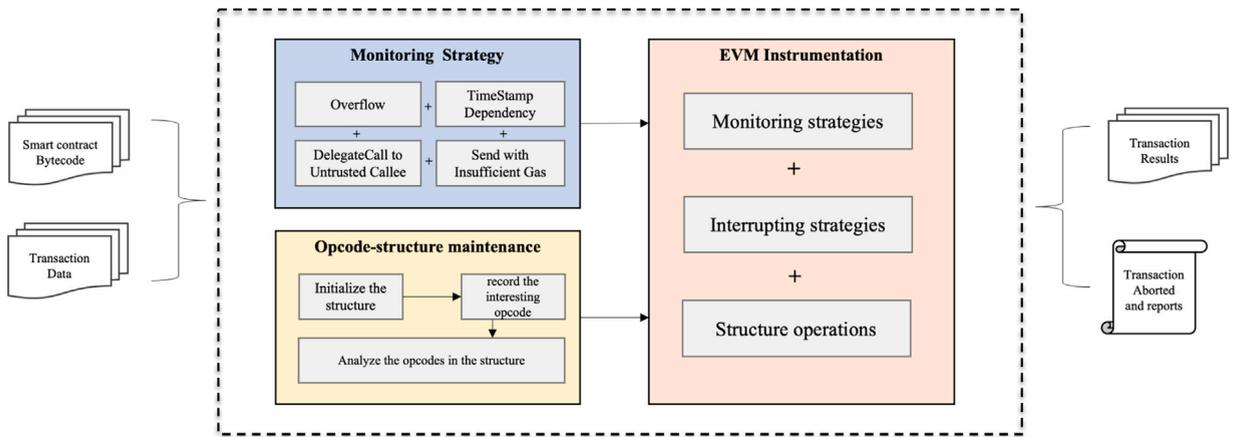
Fig. 2. The framework of the reinforced EVM\*. It mainly consists of three components: Monitoring strategy for run-time bug detection, Opcode-structure maintenance for operation monitoring, and EVM instrumentation for transaction decision and protection. The output of the virtual machine is either the transaction results or the aborted report of the dangerous transaction.
