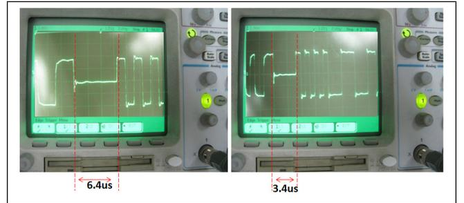
Fig. 9. We use oscilloscope to test the result that we get from the monitor. The left is the system for the GPIO operation which is 6.4us, and the right for the hardware interrupt and higher access priority one which is 3.4us.
